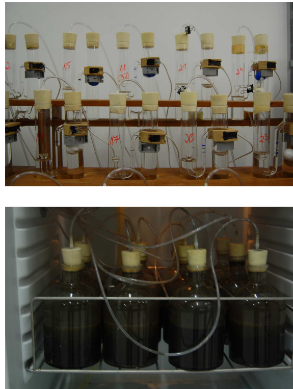
Fig. 2 Bioreactors and equipment used to collect gas.
